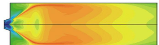
Flue Gas Temperature Distribution of Competitor's Burner
